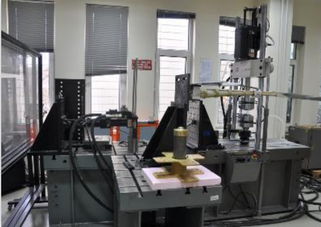
MTS testing frame: dynamical and statical testing
