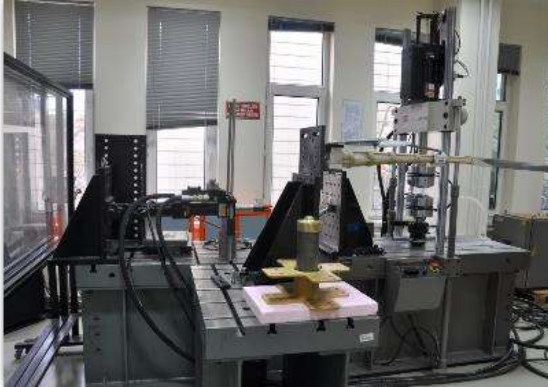
MTS testing frame: dynamical and statical testing
