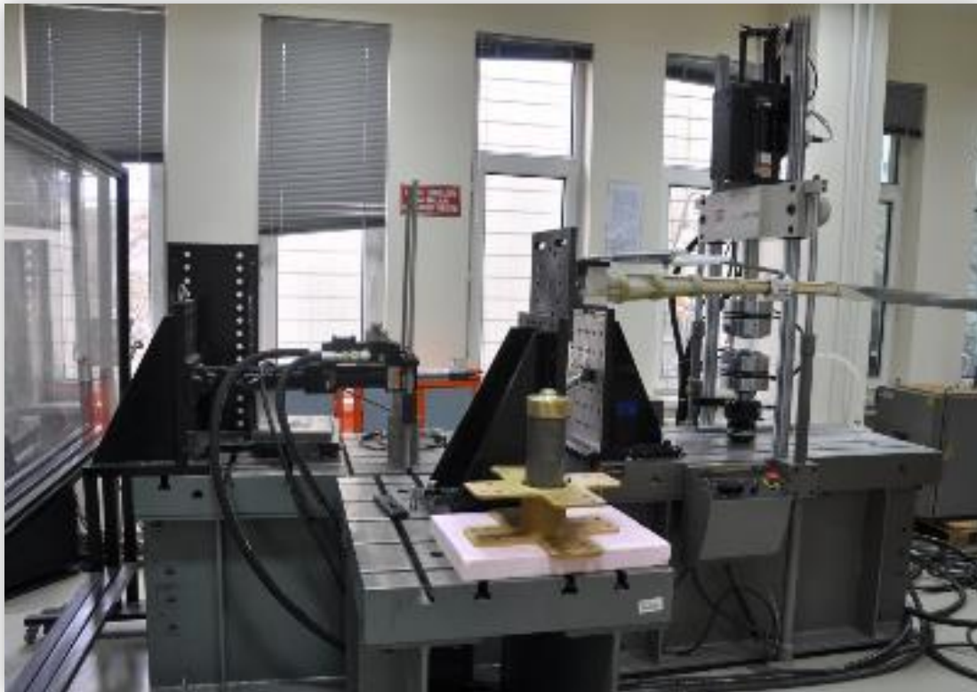
MTS testing frame: dynamical and statical testing
