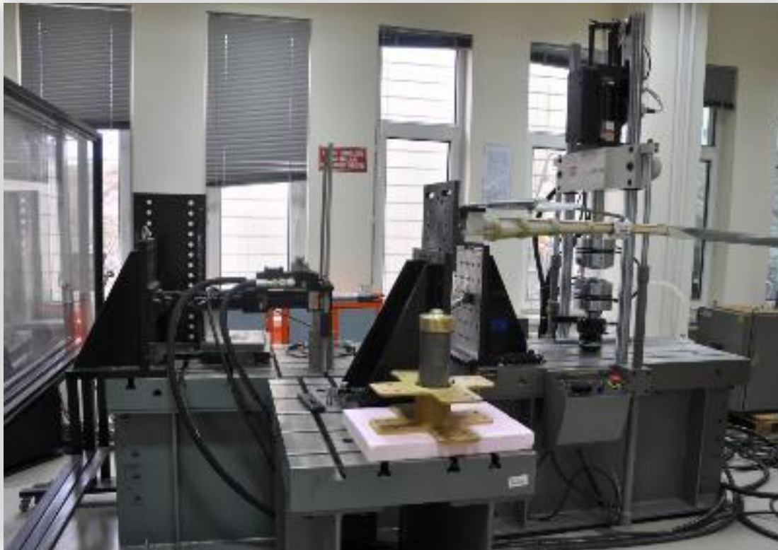
MTS testing frame: dynamical and statical testing
